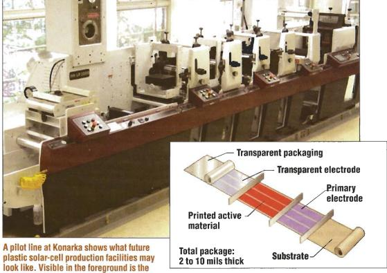
unwind station in which blank rolls are loaded. The four stations in the middle apply functional coatings. The right side has a spool at the top and one below (not visible) that are part of the apparatus for laminating and encapsulating cells. There is a via created through the lamination film through which contacts are added for electrical leads.
